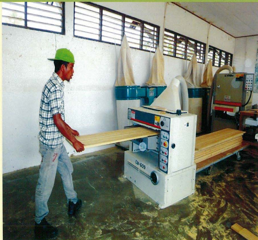
Raw- board grinding
